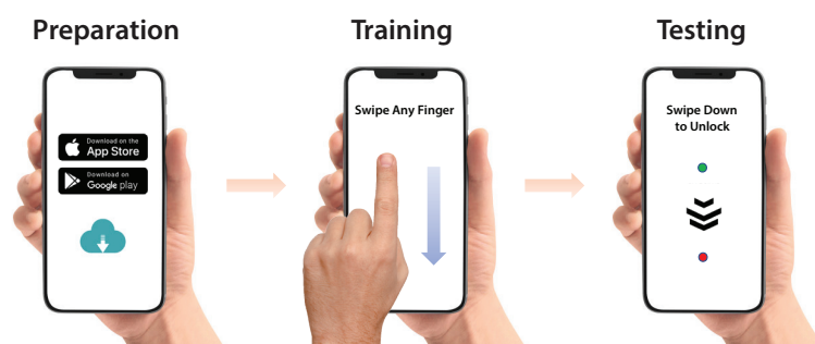
FIGURE 3. SonicPrint has a three-step deployment, with downloading the software solution, registering the biometric template and performing swipe actions, to unlock the smartphone.
